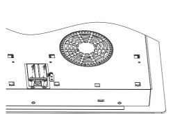
2. Remove the factory fitted cable and replace it with the 32A cable supplied for the permanent installation as per the connection diagram below. See power management on page 20, this function allow the user to select the output power total limit.
