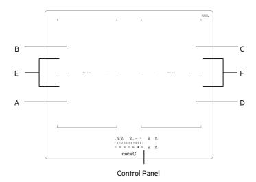
**Double Booster Heating Zone** Normal Power (W) **Booster Power (W)** Power (W) (A) Front Left Zone B Rear Left Zone © Rear Right Zone (D) Front Right Zone E Left Flexi Zone F Right Flexi Zone
